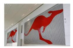
AD350 Flip-Dot Variable Message Sign is a great information or architectural feature display for indoor areas. The display can be customised to meet your specific requirements and we can provide a range of dot sizes, dot colours and custom display resolutions. Display sizes can range from small desk mounted to huge stadium display. Our driving technology is able to flip the dots in near full motion video for amazing effects.
