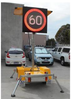
AD334 Transportable Variable Speed Limit Sign (TVSLS) is a stand-alone, solar and battery powered operated device designed for constant operation. The type C size TVSLS incorporates a 40 x 24 pixels full matrix LED display and a 5 ring LED annulus capable of displaying alpha numeric and graphic data, allowing virtually any speed and short safety instruction to be displayed (up to 3 lines of 6 characters each).
