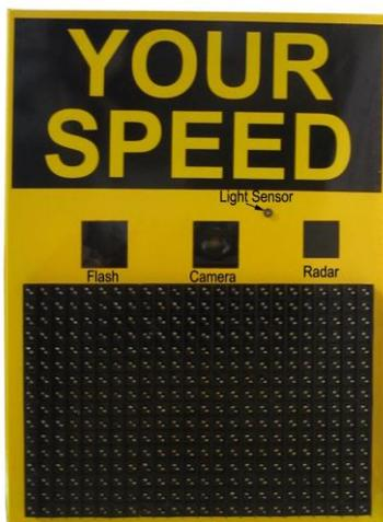
AD322 Radar Speed Displays (RSD) feature an ultra-bright LED display (24x16 pixels at 25mm pitch) integrated with radar speed sensor and data logger for traffic analysis. It provides motorists with a direct indication of their vehicle's speed and an effective trigger (message) to warn them about their speed. The radar can be set to trigger the display when vehicles are above the set limit. Ranges can be set with different responses message (up to 2 lines of 4 characters can be displayed).
