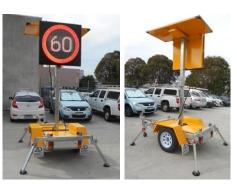
**AD334 Transportable Variable Speed Limit Sign (TVSLS)** is a stand-alone, solar and battery powered operated device designed for constant operation. The type C size TVSLS incorporates a 40 x 24 pixels full matrix LED display and a 5 ring LED annulus capable of displaying alpha numeric and graphic data, allowing virtually any speed and short safety instruction to be displayed (up to 3 lines of 6 characters each).
